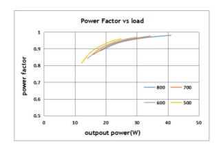
IT FIT 40 CS L Typical Power Factor vs. Load
